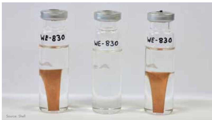
Figure 6: GTL-based transformer oils can be used alongside traditional oils. The photo shows a blend of Shell Diala S4 ZX-I (GTL) after 164 hours at 100°C: left: aged with copper and sealed, centre: aged without copper, right: aged with copper and unsealed.
