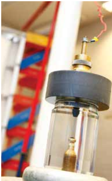
FIGURE 2: The needle-sphere electrode configuration used for lightning impulse breakdown testing.
