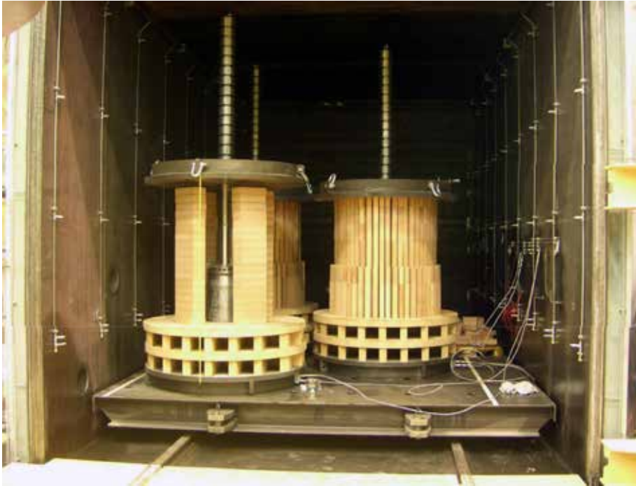
Fig. 7. Pressing tools in vapour phase oven during commissioning
