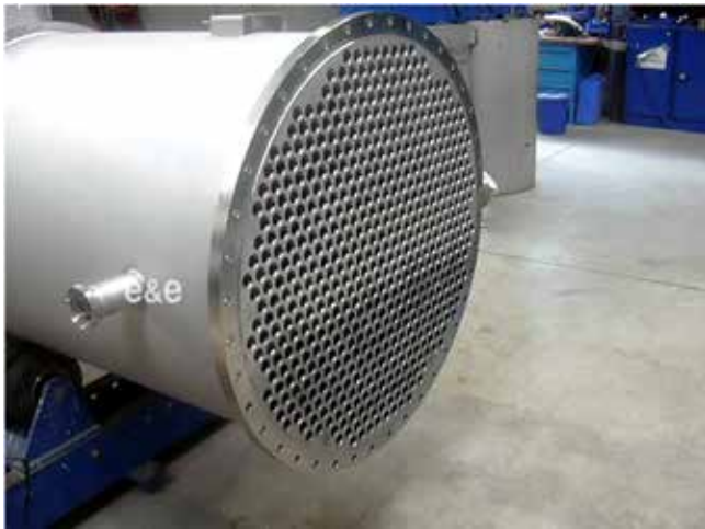
Fig. 5. View to the base plate of the evaporator showing the numerous small pipes inside
