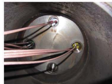
Figure 14 View on Measurement Bushings from Inside the Vacuum Oven
